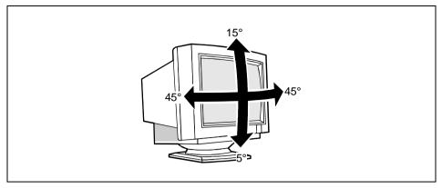
Tilting and turning area: The specified tilting area refers to the zero position of the monitor foot marked with an arrow.
