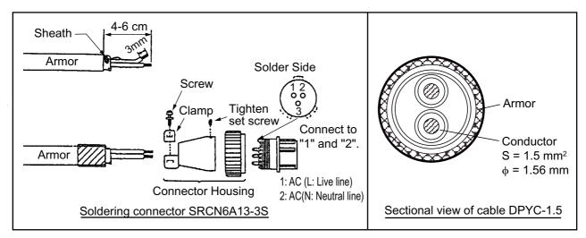
How to solder connector SRCN6A13-3S; sectional view of cable DPYC-1.5
