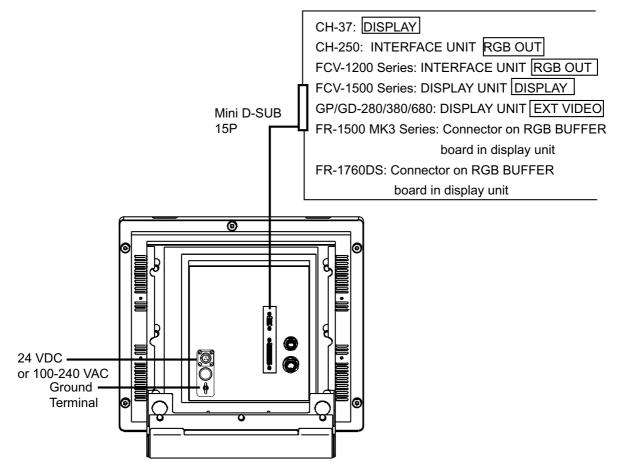
Display unit, rear view, wiring using general-purpose cables
