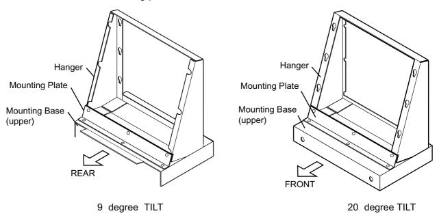
Fastening bracket and mounting plate to mounting base (upper)
