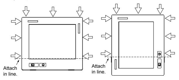
Display unit, how to attach Velcro tapes
