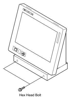
Fastening the mounting base (lower) to the display unit
