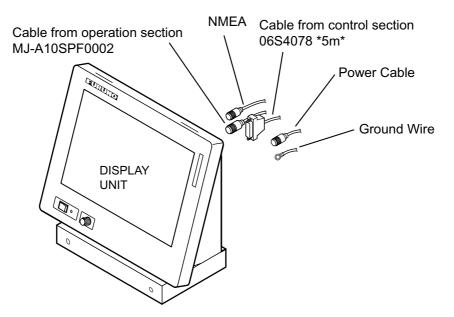
Connection of cables at the rear of the display unit
