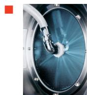
A **Rapid Jetspray Rinse** saves nearly three minutes on every rinse step! The spray rinse pulls water through linens, allowing it to drain immediately, rather than cycling through the time-consuming fill, agitation and drain phases of the traditional bath rinse.
