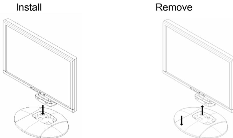
Figure 1 Installing and Removing the Base
