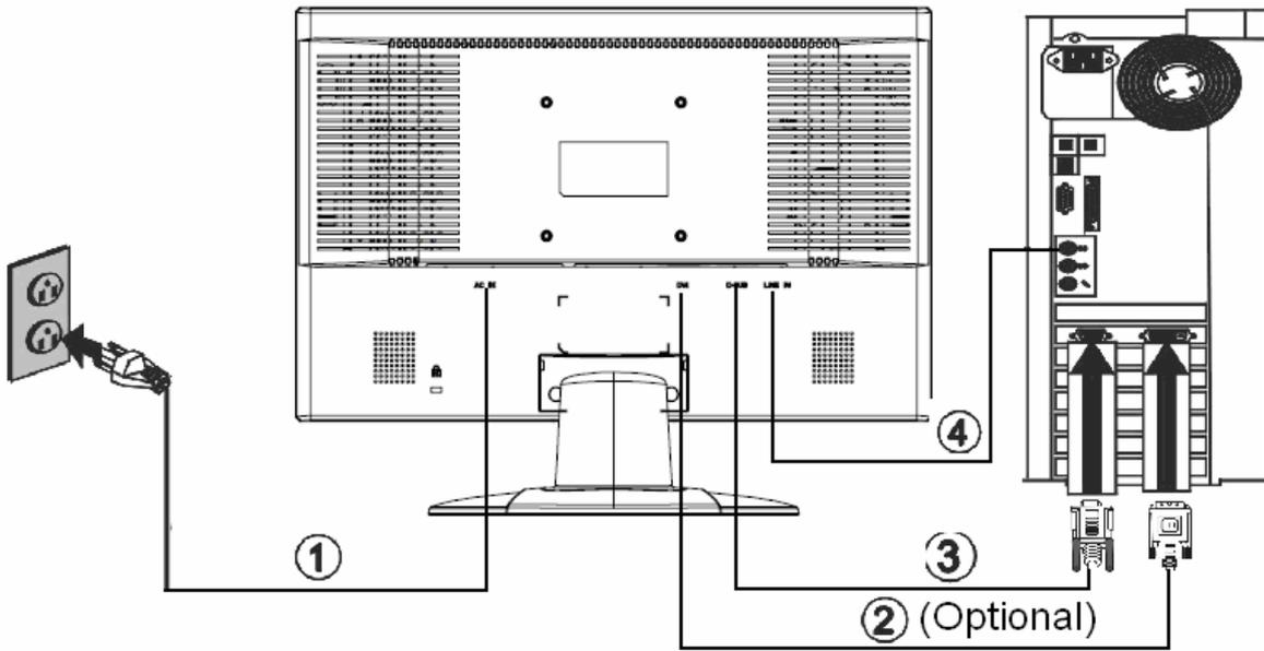
Figure 2 Connecting Cables
