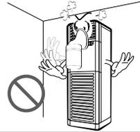
**When flammable gas leaks, turn off the gas and open a window for ventilation before turn the product on.**
