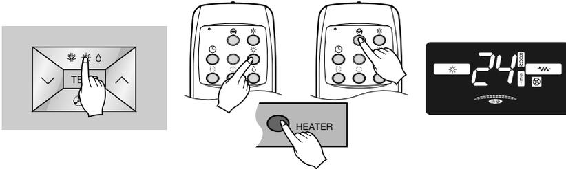
**3** Set the temperature upper than the room temperature. The temperature can be set within a range of 16°C~30°C by 1°C.
