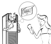
When the product is not be used for a long time, disconnect the power supply plug or turn off the breaker.
