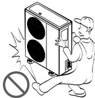
Do not install the product where it will be exposed to sea wind (salt spray) directly.
