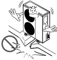
**Be sure the installation area does not deteriorate with age.**
