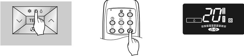
**3** Set the temperature lower than the room temperature.
