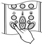
□ Each time the Button is pressed, the Fan Speed mode is shifted.
