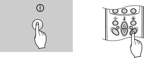
**2** Select heating Operation by pressing the Operation Mode Selection button. Press the Heater Operation Button on the remote controller.
