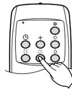
Press the Airflow Direction Control Button again to set the Vertical louver at the desired airflow direction.
