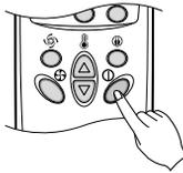
**2** Press the **Jet Cool** button to operate the speed cooling mode and the unit will operate in high fan speed on cooling mode.
