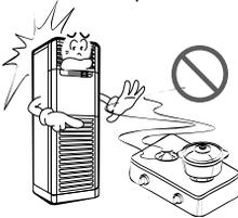
**If strange sounds, or small or smoke comes from product. Turn the breaker off or disconnect the power supply cable.**
