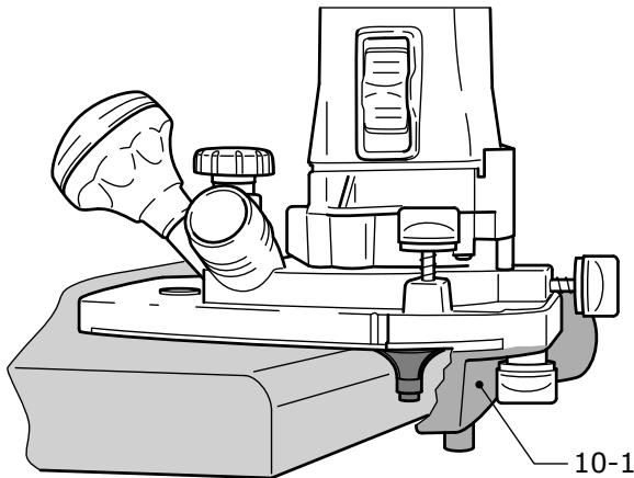
Use routing tools with a bearing guide in the machine when edge trimming with the large surface router table. The machine is then guided in such a way that the bearing guide rolls off the workpiece.
