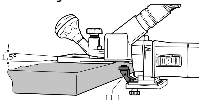
When edge trimming with the router table for edge veneer (only in SET scope of delivery), fit the sensor [11-1] to the machine (see "Router table for edge veneer"). The machine is then guided in such a way that the sensor rests against the workpiece.
