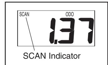
To select only the Speed, Distance, Time, Odometer, or Calorie mode, press the console button until only the SPEED, DIST, TIME, ODO, or CAL indicator appears in the display. Make sure that the SCAN indicator does not appear.
