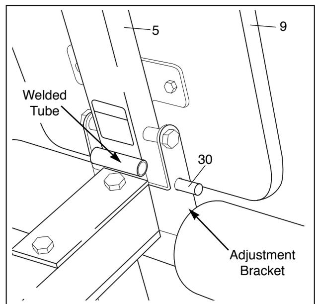
**WARNING:** When the seat is tilted to the upright position, always insert the locking pin into the hole in the seat frame as shown. Do not insert the locking pin into the welded tube.
