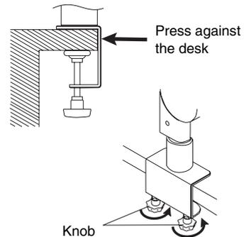
Use specified screws for tightening up referring to the 'Compatible Screws List'.
