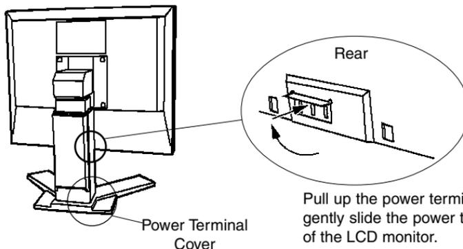
Pull up the power terminal cover with your finger, and gently slide the power terminal cover into the groove of the LCD monitor.
