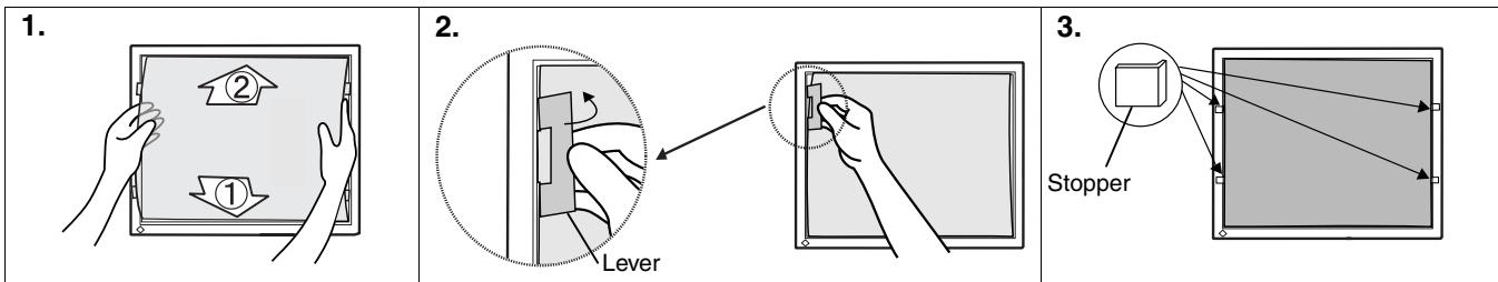
**1. Set the panel protector into the grooves of the panel frame; the lower first (1), then the upper (2).**
