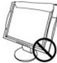
Blocking the ventilation slots prevents proper airflow and may result in fire, electric shock, or equipment damage.
