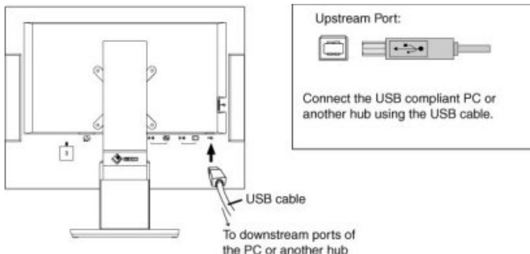
After connecting the USB cable, the USB function can be set up automatically.
