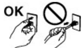
**The equipment must be connected to a grounded main outlet.**
