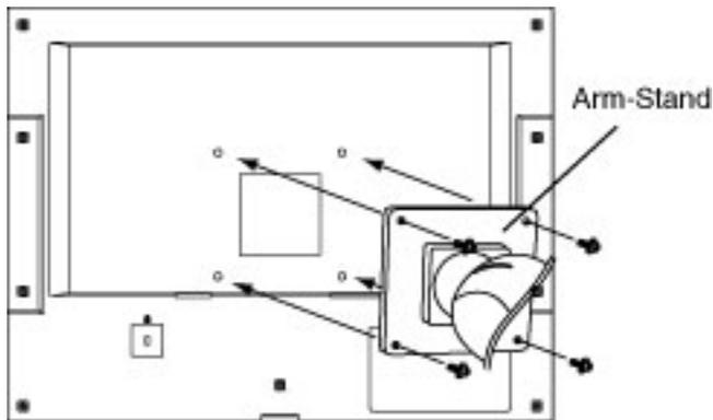
4 Mounting Screws (enclosed): M4 x 12 mm
