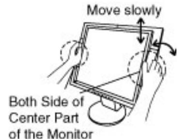
**(1) Adjust the height of the monitor. To heighten, push the monitor backward. To lower, pull the monitor forward.**
