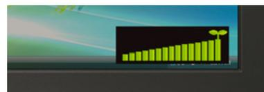
*When EcoView Index is fully illuminated, the monitor is operating at optimum energy efficiency.*
