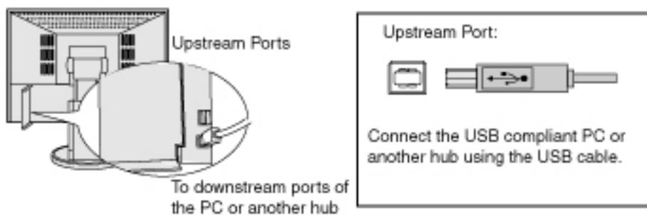
After connecting the USB cable, the USB function can be set up automatically.
