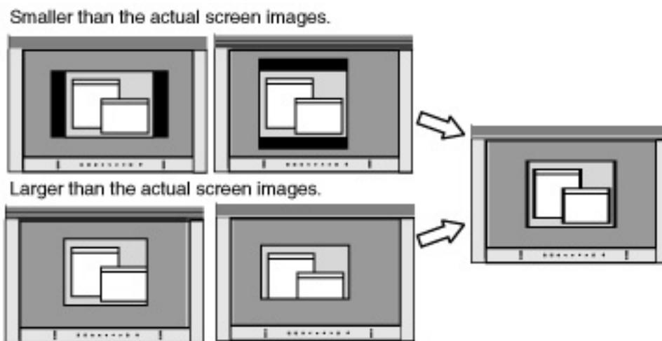
**4.Adjust the output signal range (Dynamic Range) of the signal.**
