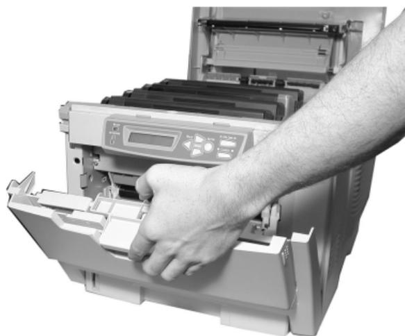
5. Lift up on the ends and remove the side panel from the printer.
