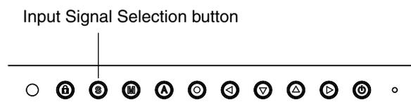
The monitor recognizes the connector through which PC signals are input. When either PC is turned off or enters the power-saving mode, the monitor automatically displays signals of another PC.
