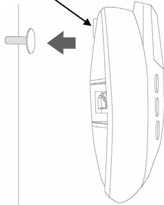
2. Align nails or picture hooks with the wall-mount hanger located on the bottom surface of the base.
