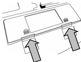
2. Carefully install three (3) AAA batteries by observing the polarity direction shown in the battery compartment.
