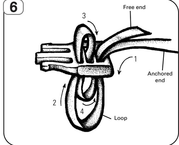
**To tighten waist belt**, feed the anchored end of the waist belt up through the buckle to form a loop. Pull the free end of the waist belt through.
