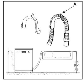
The pipe should not be immersed in water.
