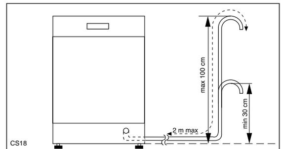
Likewise the internal diameter of the couplings used for connections to the waste outlet must be no smaller than the diameter of the hose provided.
