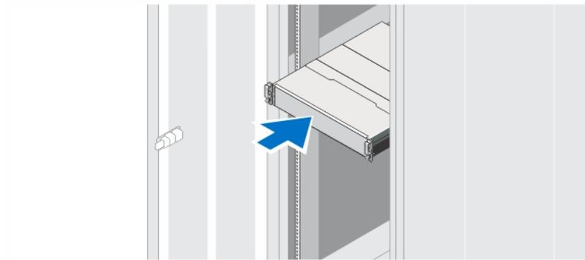
**Figure 1. Installing the System in a Rack**
