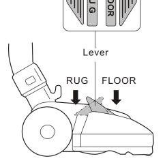
This rug attachment has a small, built-in turbine that is driven by the suction force of the unit. The turbine drives a brush inside the attachment to pick up fine particles more efficiently.
