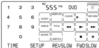
To change the Label keys, press the Mode Display key (in this case, DVD) repeatedly. Each time you press the DVD key, the display of the Label keys changes as follows.
