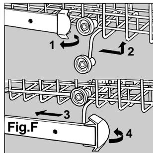
Open the rail stop flaps and pull the basket out completely. Now place it in high or low position, then slide it along the guide rails until the front wheels also go in. Now close the rail stop flaps. Follow the sequence of actions illustrated in figure "F".
