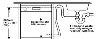
**NOTE:** Ensure the sink outlet pipe has a minimum diameter of 32mm.
