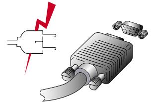
1. Insert the other 15-pin/DVI-D signal cable connector into the 15-pin VGA/DVI-D connection on your computer and screw it down.
