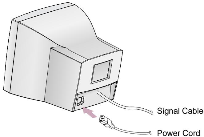
If your power cord is PC-to-Monitor type, plug the other end of the power cord into the AC receptacle in the computer.
