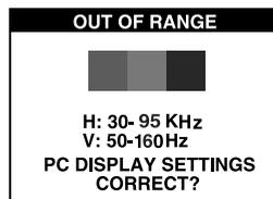
Out of Range screen is displayed when the applied frequency is under or over normal range.
