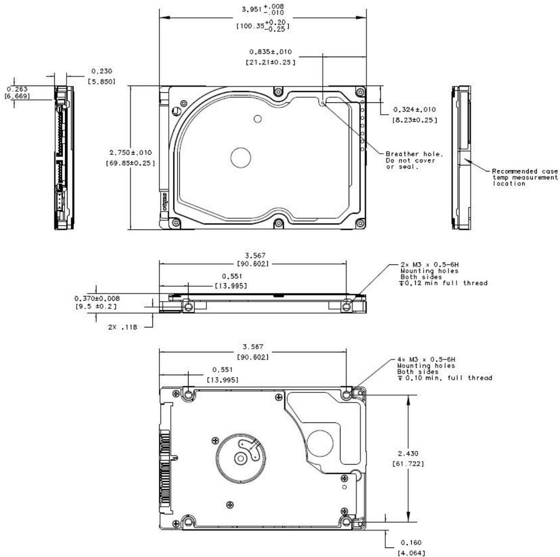
Figure 3. Mounting dimensions—top, side and end view
