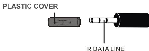
This 3.5Φ IR Jack has plastic cover to prevent short, to remove the plastic cover, please do not pull it out directly, please rotate the plastic cover and put it out slowly.
