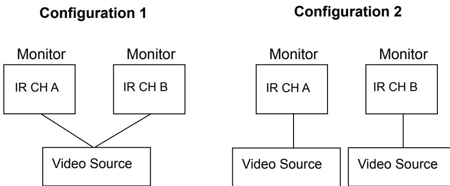
If two monitors are used for rear entertainment systems, dual channel wireless headphones (WH253H) are most appropriate. In this circumstance, channels A and B on both headphone and monitor should be set respectively.
