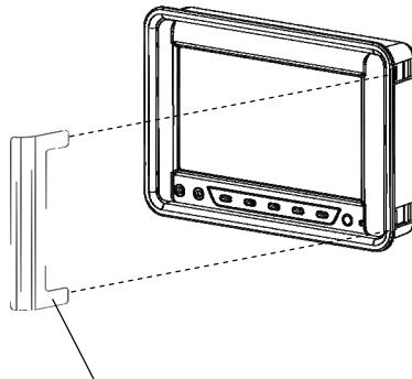
[Insert the metal insert card to take monitor out of the bezel](#)
