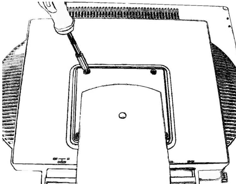
**Figure 6.1** Removing the Base
