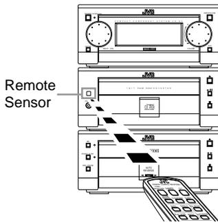
When using the remote control, point it at the remote sensor on the front panel.
