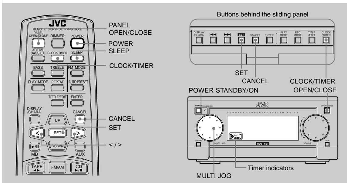
On FS-G6 system, three timer features are available — Recording Timer, Daily Timer, and Sleep Timer. Before using these timers, you need to set the clock built in the system (see page 10).
