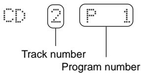
Here the track number 2 on the CD is stored into a program number 1, and shortly after that the total playback time of programmed tracks appears in the display window as follows:
