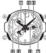
Button operations are indicated using the letters A through D shown in the illustration.
