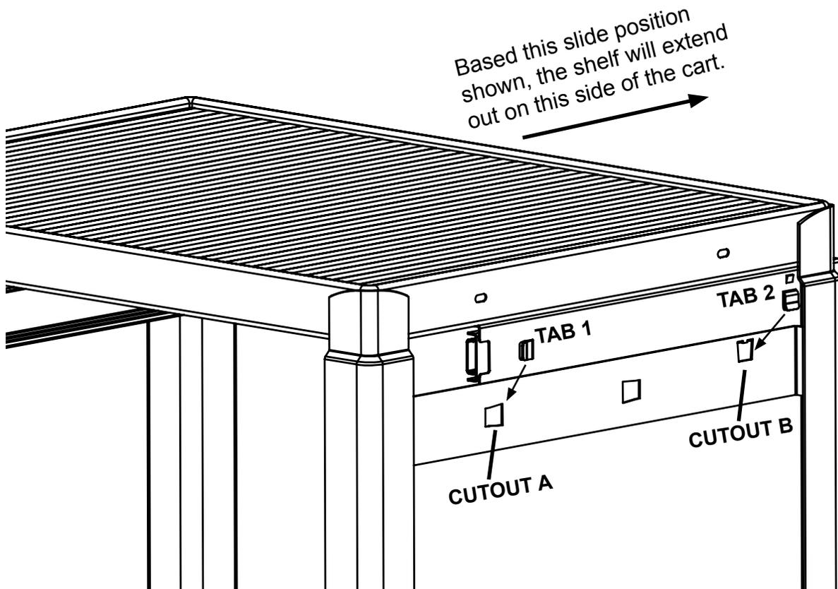
Based this slide position shown, the shelf will extend out on this side of the cart.
