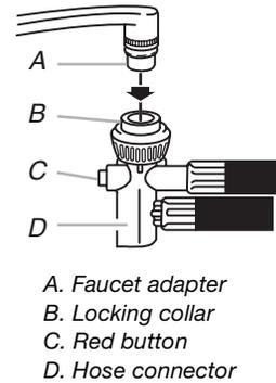
3. Lift slightly on the hose connector while pulling down the locking collar. Pull down on the connector.
