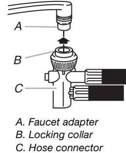
4. When the connector snaps into place, release the locking collar.
