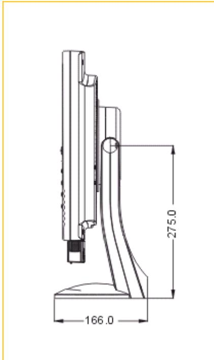
For viewing clarity, you can tilt the LCD panel forward (up to 5 degrees) or backward (up to 20 degrees)
