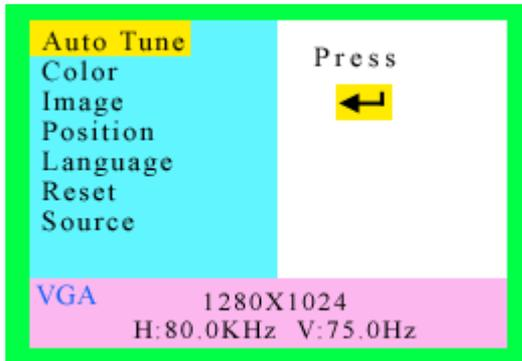
Press "←" button, the system will automatically adjust the clock, phase, H-position and V-position values for optimal settings.
