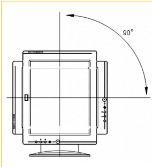
You can turn the LCD panel right 90 degree for particular viewing.
