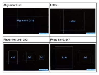
When QuickFit is activated, press the control buttons on the front panel to make adjustments. The QuickFit OSD displayed in the lower right corner of the screen will guide users to make selections.
