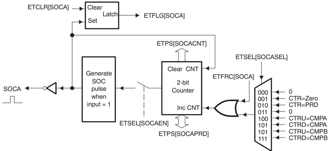
Figure 2-43 shows the operation of the event-trigger's start-of-conversion-B (SOCB) pulse generator. The event-trigger's SOCB pulse generator operates the same way as the SOCA.
