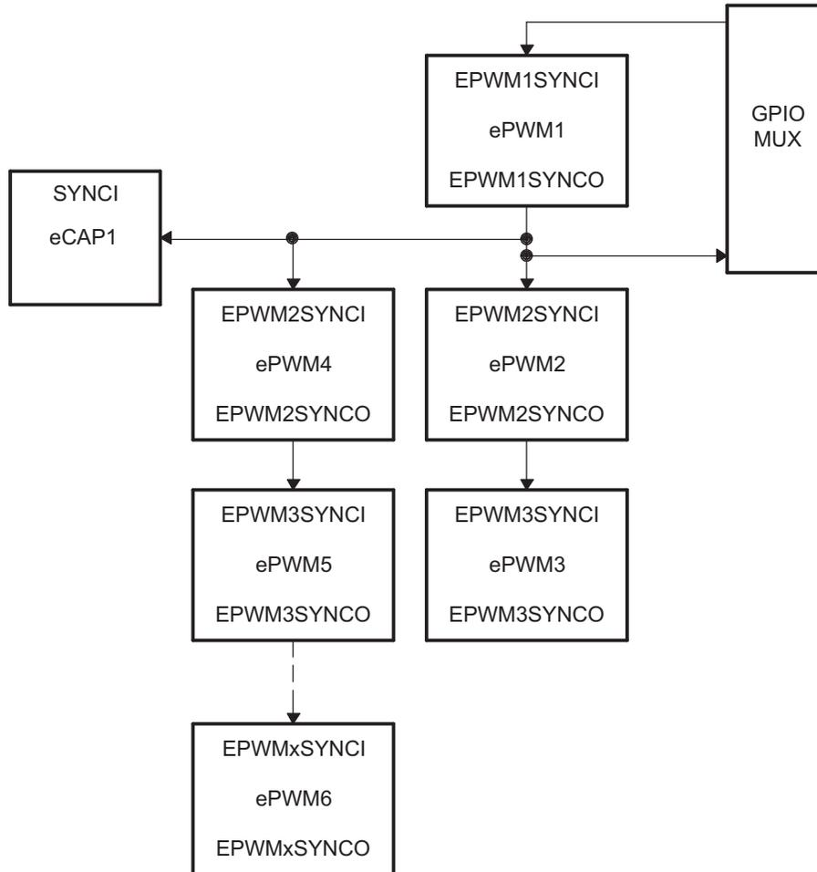
Each ePWM module can be configured to use or ignore the synchronization input. If the TBCTL[PHSEN] bit is set, then the time-base counter (TBCTR) of the ePWM module will be automatically loaded with the phase register (TBPHS) contents when one of the following conditions occur:
