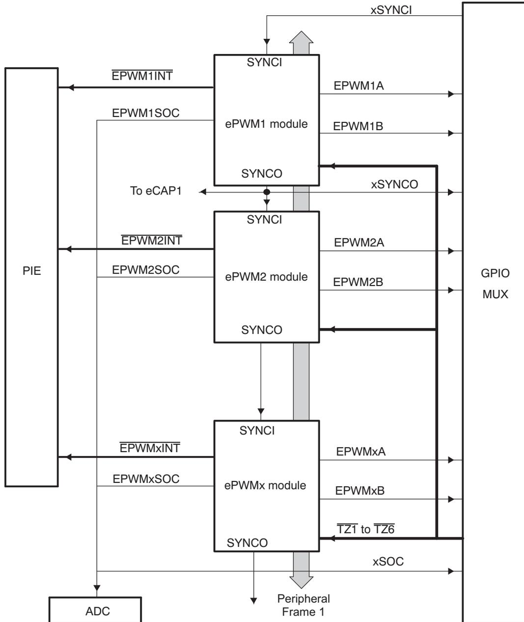
The order in which the ePWM modules are connected may differ from what is shown in [Figure 1-1](#). See [Section 2.2.3.2](#) for the synchronization scheme for a particular device. Each ePWM module consists of seven submodules and is connected within a system via the signals shown in [Figure 1-2](#).
