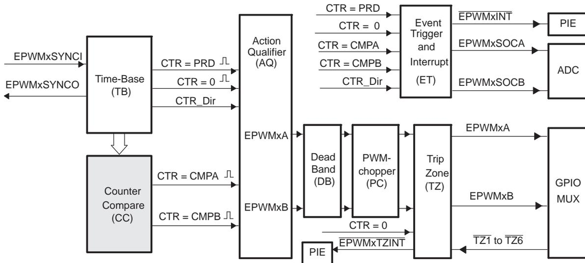
Figure 2-12 shows the basic structure of the counter-compare submodule.
