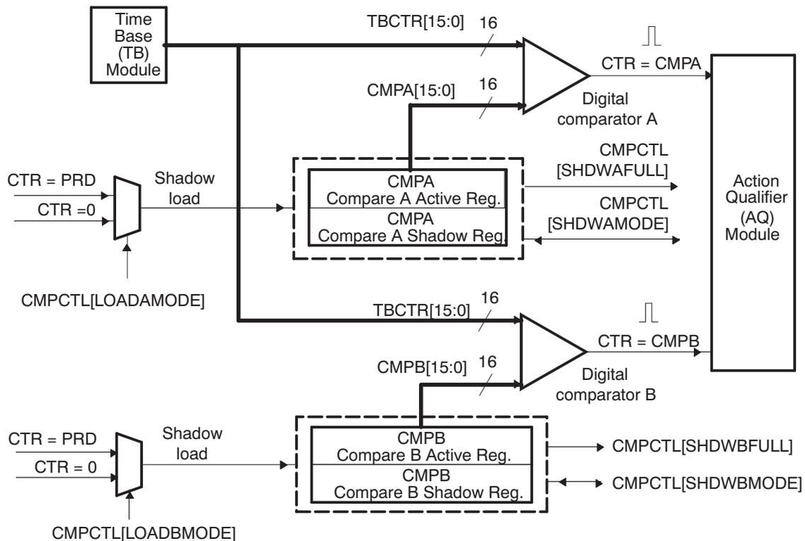
The key signals associated with the counter-compare submodule are described in [Table 2-5](#).
