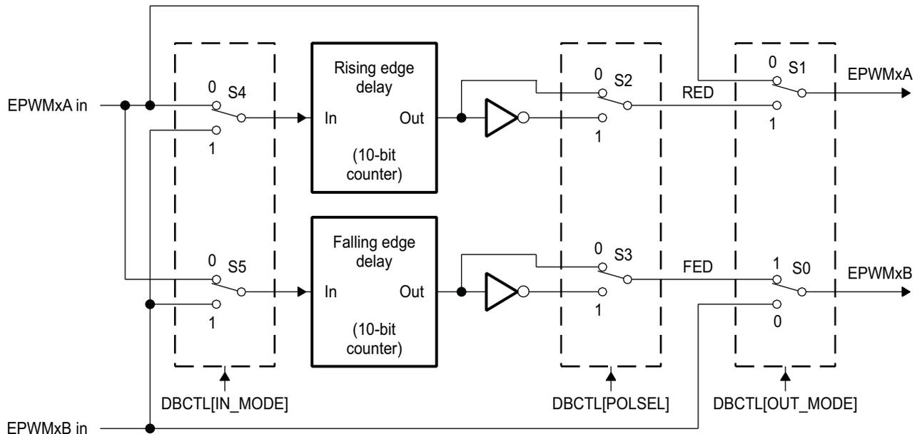
Although all combinations are supported, not all are typical usage modes. [Table 2-13](#) documents some classical dead-band configurations. These modes assume that the DBCTL[IN\_MODE] is configured such that EPWMxA In is the source for both falling-edge and rising-edge delay. Enhanced, or non-traditional modes can be achieved by changing the input signal source. The modes shown in [Table 2-13](#) fall into the following categories:
