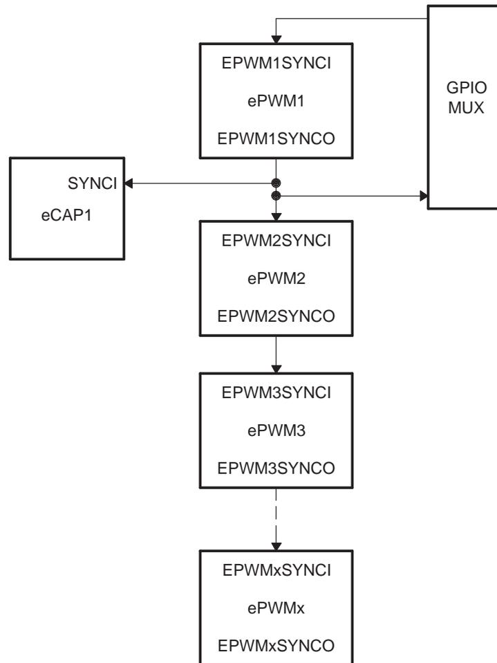
Scheme 2 shown in [Figure 2-5](#) is used by the 2804x devices when the ePWM pinout is configured for A-channel only mode (GPAMCFG[EPWMMODE] = 3). If the 2804x ePWM pinout is configured for 280x compatible mode (GPAMCFG[EPWMMODE] = 0), then Scheme 1 is used.
