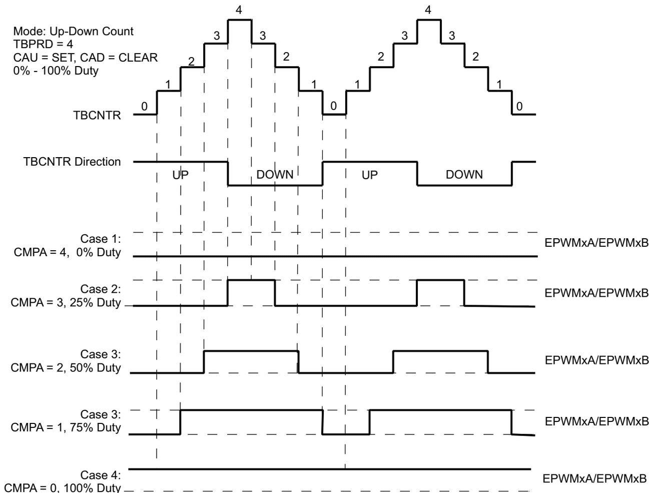
The PWM waveforms in [Figure 2-21](#) through [Figure 2-26](#) show some common action-qualifier configurations. The C-code samples in [Example 2-2](#) through [Example 2-7](#) shows how to configure an ePWM module for each case. Some conventions used in the figures and examples are as follows:
