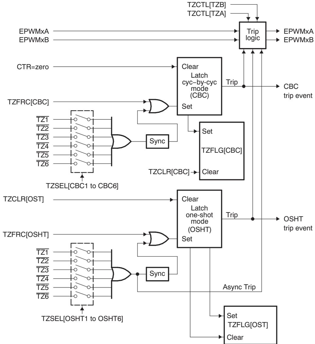
**Figure 2-37. Trip-Zone Submodule Interrupt Logic**
