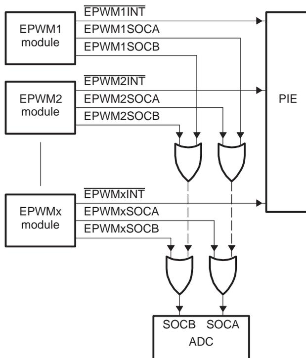
The event-trigger submodule monitors various event conditions (the left side inputs to event-trigger submodule shown in Figure 2-40) and can be configured to prescale these events before issuing an Interrupt request or an ADC start of conversion. The event-trigger prescaling logic can issue Interrupt requests and ADC start of conversion at:
