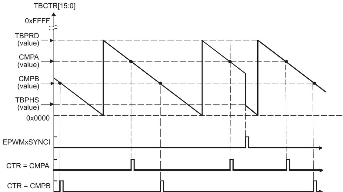
**Figure 2-15. Counter-Compare Events In Up-Down-Count Mode, TBCTL[PHSDIR = 0] Count Down On Synchronization Event**
