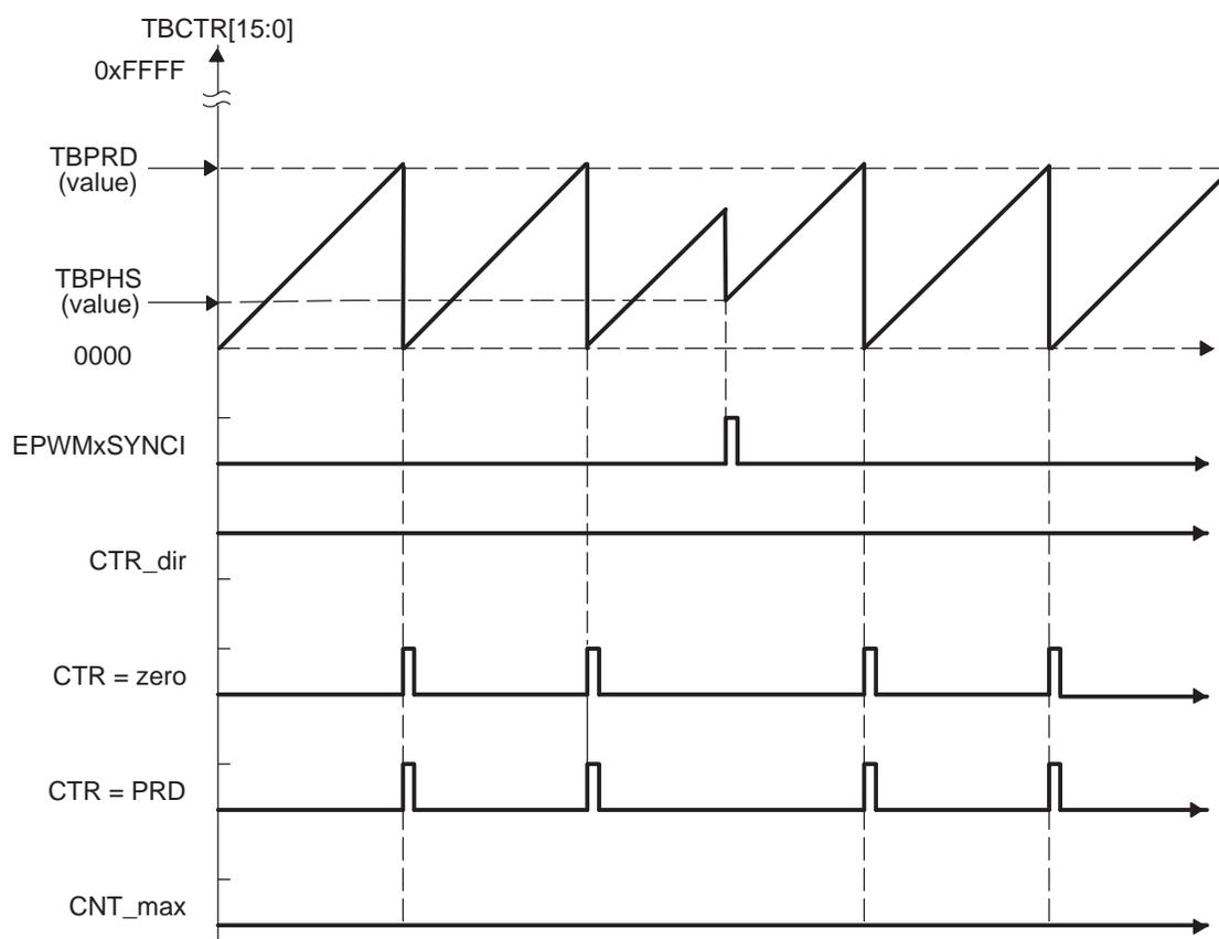
**Figure 2-8. Time-Base Down-Count Mode Waveforms**
