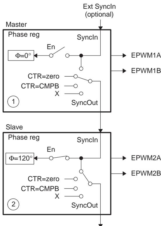
[Figure 3-12](#) shows the associated timing waveforms for this configuration. Here,  $TBPRD = 600$  for both master and slave. For the slave,  $TBPHS = 200$  (i.e.,  $200/600 \times 360^\circ = 120^\circ$ ). Whenever the master generates a SyncIn pulse ( $CTR = PRD$ ), the value of  $TBPHS = 200$  is loaded into the slave TBCTR register so the slave time-base is always leading the master's time-base by  $120^\circ$ .
