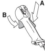
Make sure the throttle control is locked at the idle setting when the throttle lockout is released.
