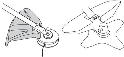
Check that the guard is undamaged and not cracked. Replace the guard if it has been exposed to impact or is cracked.
