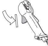
Press the throttle lockout and make sure it returns to its original position when you release it.
