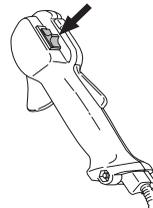
**CAUTION!** The stop switch automatically returns to the start position. In order to prevent unintentional starting, the spark plug cap must be removed from the spark plug when assembling, checking and/or performing maintenance.
