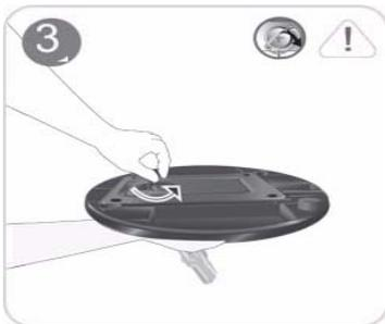
Turn the connecting screw at the bottom of the stand to separate it.
