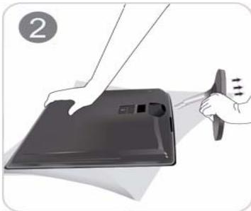
Hold the main body of the product with your hand as shown by the figure. Pull the stand in the direction of the arrow as shown in the figure to separate it.
