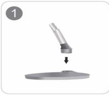
Insert the Stand Connector into the Stand in the direction shown by the figure.
