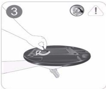
Turn the connecting screw at the bottom of the stand fully so that it is completely fixed.
