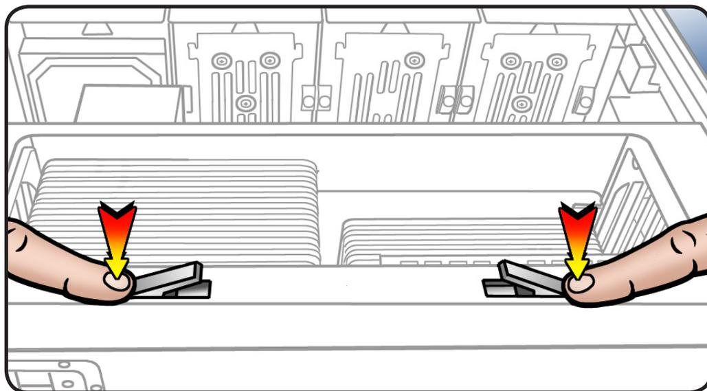
**3** Holding tray by latches, lift it out of computer.
