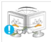
▶ Do not lift or move the product back and forwards or right and left while only holding the power cord or signal cables.
