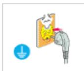
▶ Make sure to connect the power cord to a grounded power outlet.
