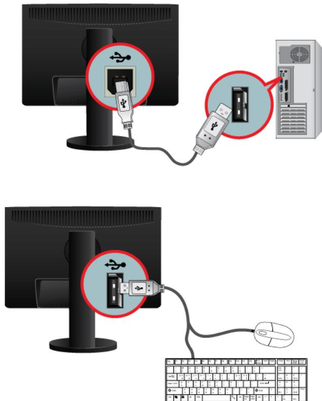
1. Connect the
