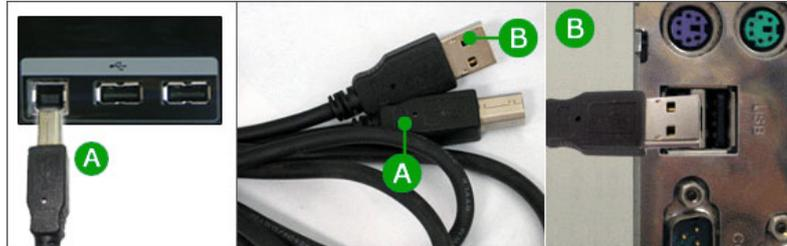
2. Connect the
