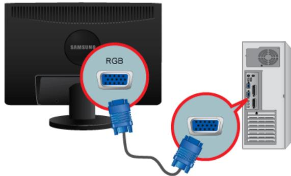
**1** Using the D-sub (Analog) connector on the video card.
