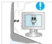
▶ Install your product in a well ventilated location. Ensure that there is a clearance of more than 10 cm from the wall.
