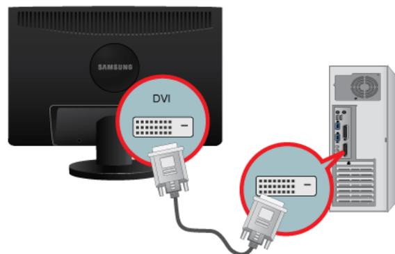
**2** Using the DVI (Digital) connector on the video card.
