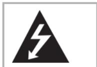
This symbol indicates that dangerous voltage constituting a risk of electric shock is present within your radio. This label is located on the back of your radio.
