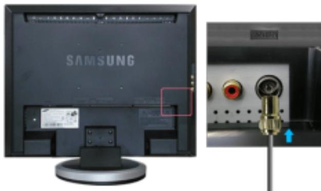
1. Connect the CATV cable or TV antenna cable to the "ANT IN" port on the rear side of the monitor. Make sure to use a TV antenna cable (sold separately) as the antenna cable.
