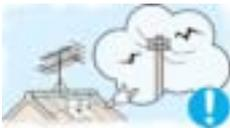
❗ **If you are using an outdoor antenna, be sure to put sufficient distance between your antenna and the electrical wires nearby so that they would not come in contact with each other in case the antenna is knocked over by strong wind.**
