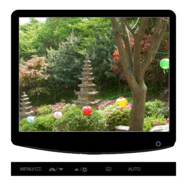
When the 'AUTO' button is pressed, the auto adjustment screen appears as shown in the animated screen on the center.
