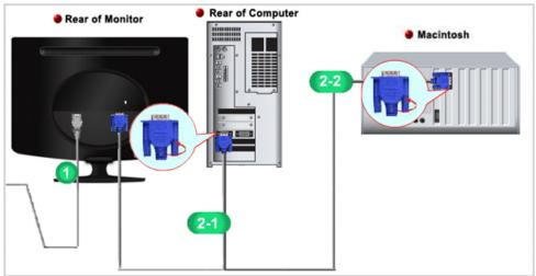
1 Connect the power cord for your monitor to the power port on the back of the monitor.
