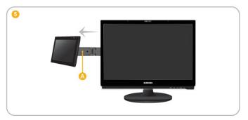
5. When disassembling the 7" USB monitor, remove it by holding the A part and pushing it in the direction of the arrow.
