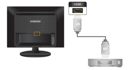
1. Input devices such as digital DVD are connected to the *HDMI* terminal of the monitor using the HDMI cable. When all the connections are completed, connect the power cords for the monitor and DVD (or the device connected to the digital output terminal).
