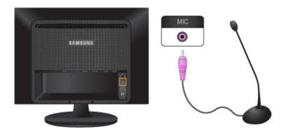
1. Connect the microphone cable to the MIC port on the monitor.
