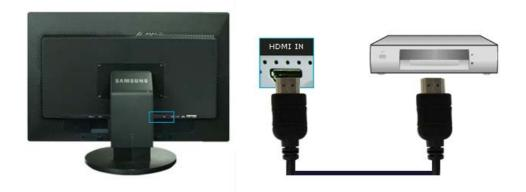
0 Input devices such as digital DVD are connected to the HDMI IN terminal of the monitor using the HDMI cable. When all the connections are completed, connect the power cords for the monitor and DVD (or the device connected to the digital output terminal). Select HDMI using the 'source' button.
