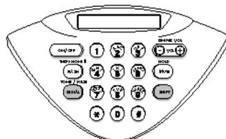
To access digital services, such as voice mail, where only pulse dialing is available, SoundStation Premier can provide temporary tone dialing. When the phone is **ON**, press **SHIFT**, then press **REDIAL**. The display must read **TONE DIALING** for this feature to be activated. Once the phone is hung up, dialing will revert to its previous mode.
