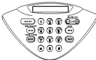
To access digital services, such as voice mail, where only pulse dialing is available, SoundStation Premier can provide temporary tone dialing. When the phone is **ON**, press **SHIFT**, then press **REDIAL**. The display must read **TONE DIALING** for this feature to be activated. Once the phone is hung up, dialing will revert to its previous mode.
