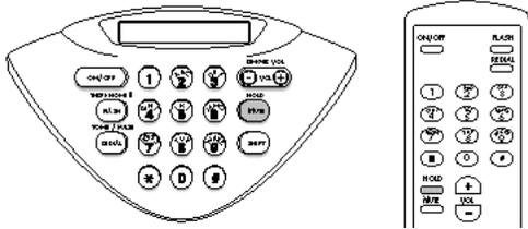
To take the phone off **HOLD** press only the **MUTE** key on the main keypad or **HOLD** on the remote keypad. To shut off the microphones while keeping the speaker on, simply press **MUTE**.
