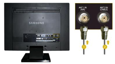
If your antenna has a set of leads that look like the diagram to the right, see "Antennas with 300  $\Omega$  Flat Twin Leads" below.
