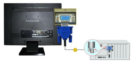
1. Using the D-sub (Analog) connector on the video card. Connect the signal cable to the D-SUB port on the Macintosh computer. 6(.....)6 [PC]
