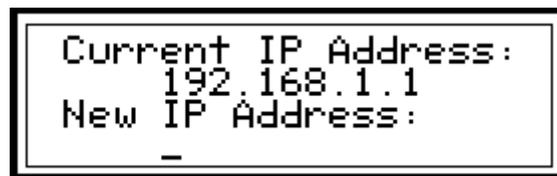
Figure 16- Set IP Address from LCD and keypad
