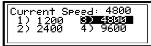
Figure 15- Set baud rate from LCD and keypad
