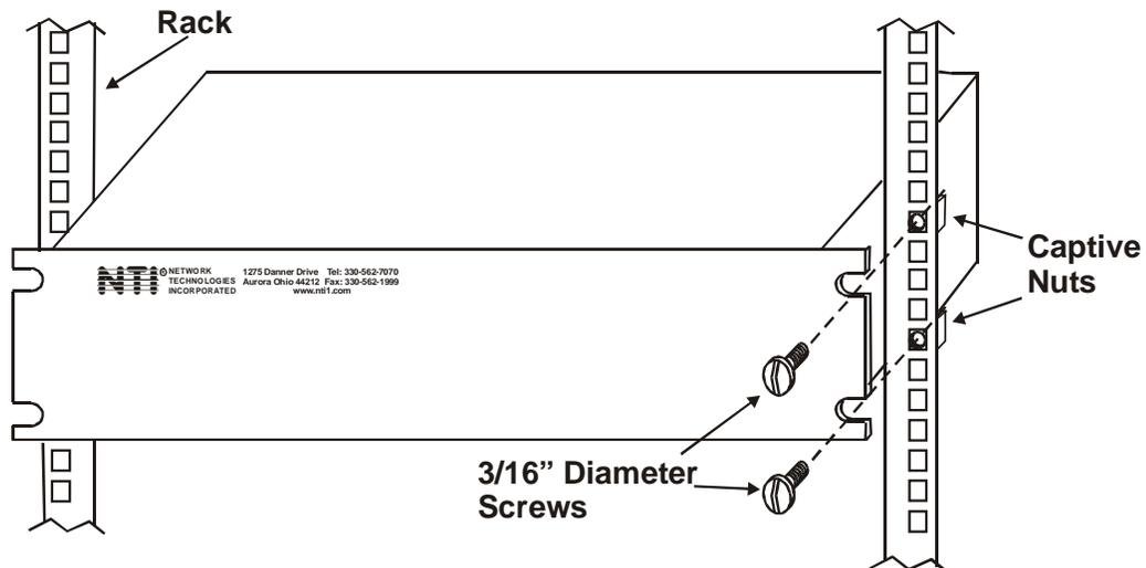
**Figure 33- Mount Switch to a Rack**
