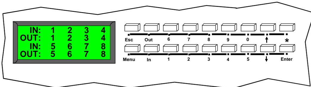
Figure 10- Front panel Interface LCD and keypad
