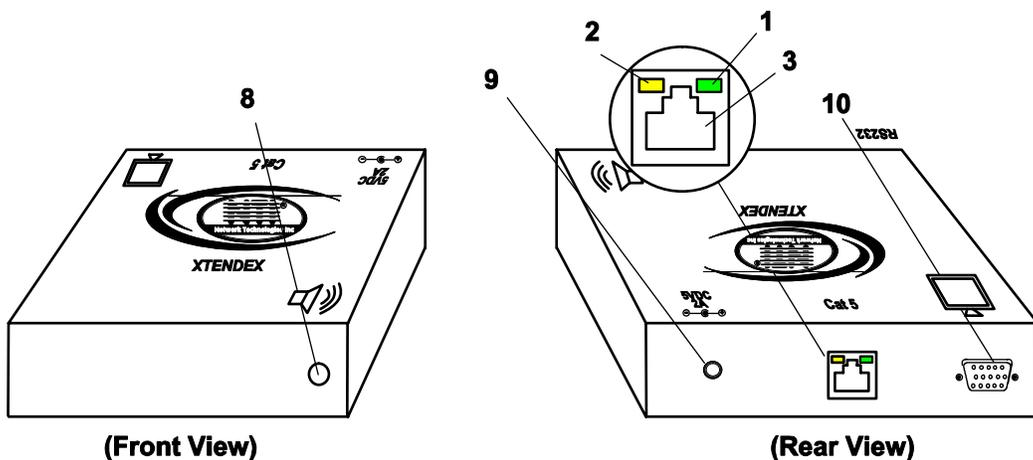
**ST-C5VA-600 Remote Unit (VGA plus Audio)
