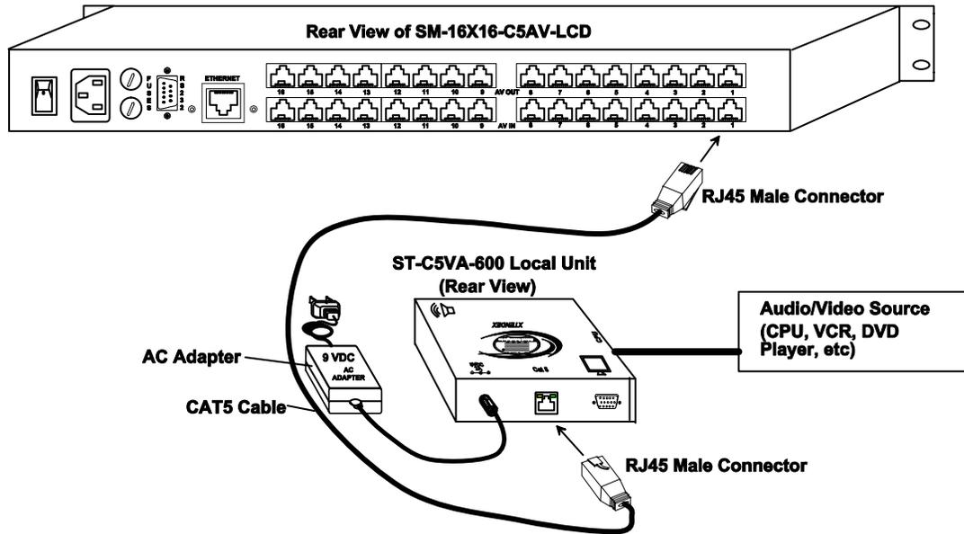
Figure 5- Attach ST-C5VA-600 Local Unit to VEEMUX
