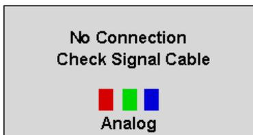
This box appears during normal operation if the video cable becomes disconnected or damaged.
