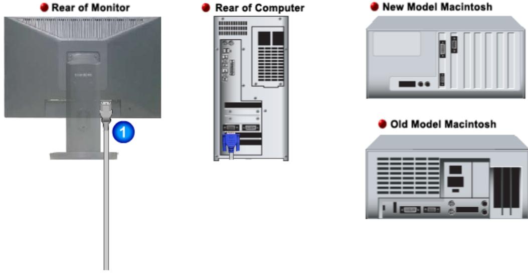
1. Connect the power cord for your monitor to the power port on the back of the monitor. Plug the power cord for the monitor into a nearby outlet.
