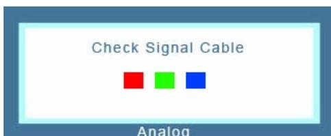
This box appears during normal operation if the video cable becomes disconnected or damaged.
